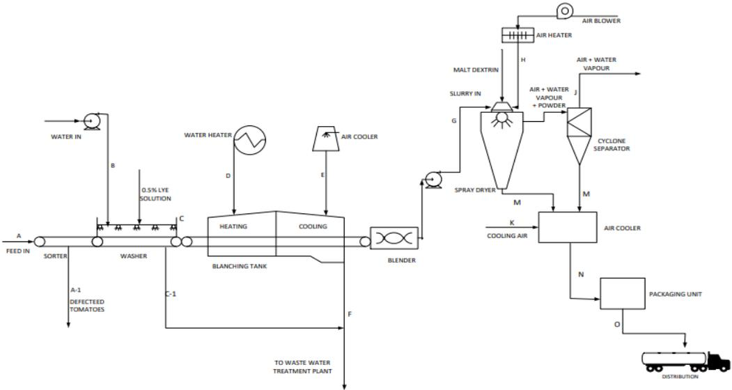
Fig. 4. Process flow diagram of tomato powder processing plant.
