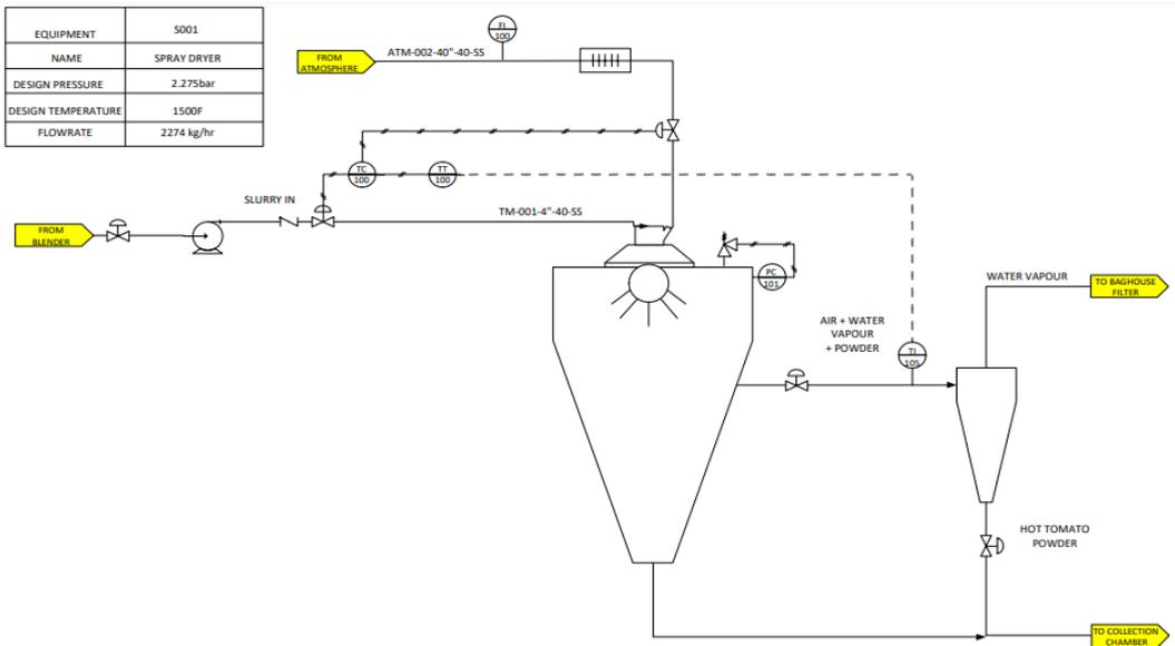
Fig. 7. Piping and instrumentation diagram of spray dryer
