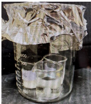
Figure 1: Simple environmental chamber for deliquescence experiments
