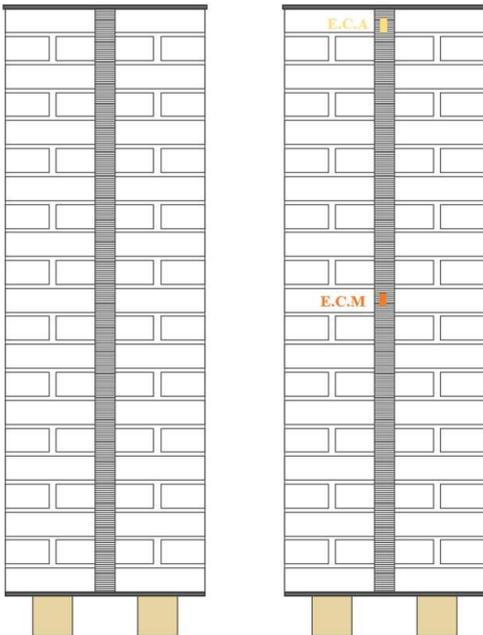
Figure 17. Instrumentation of specimen P2 with strain-gauges: compressed face on the left and stretched face on the right.
