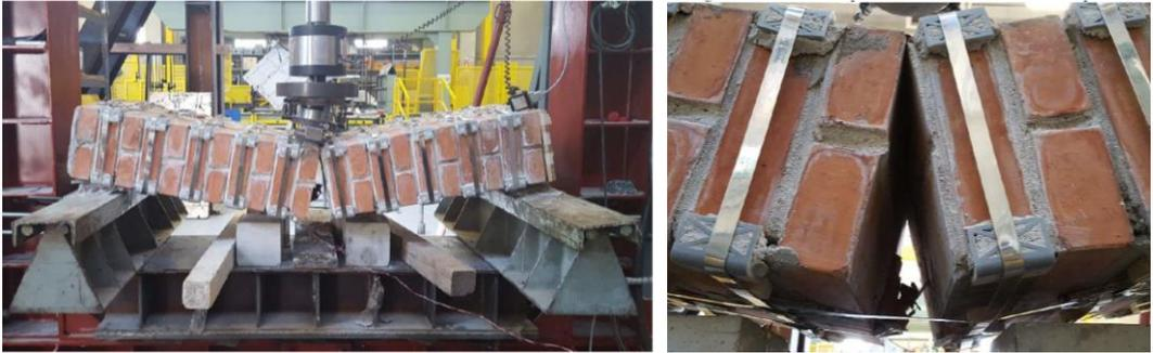
Figure 19. Deformation of the specimen P1 during bending test: zoom of the central part on the right.
