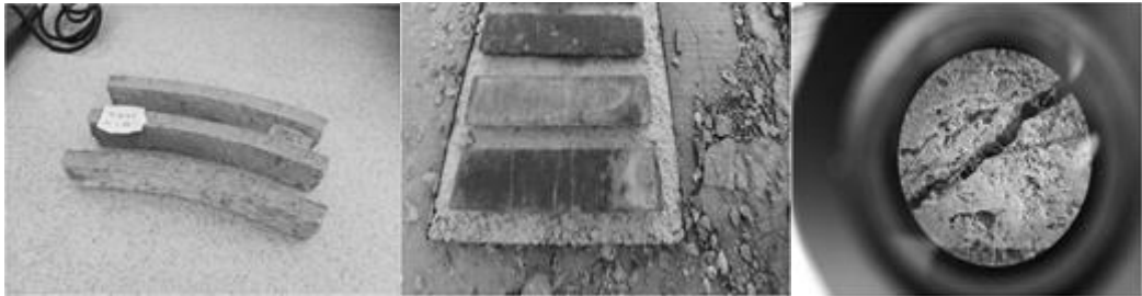
Figure 2. Small mortar beams for self-healing measurement
