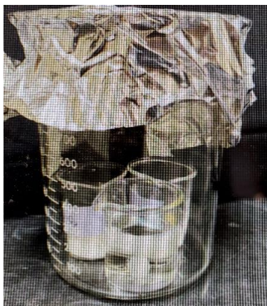
Figure 1: Simple environmental chamber for deliquescence experiments
