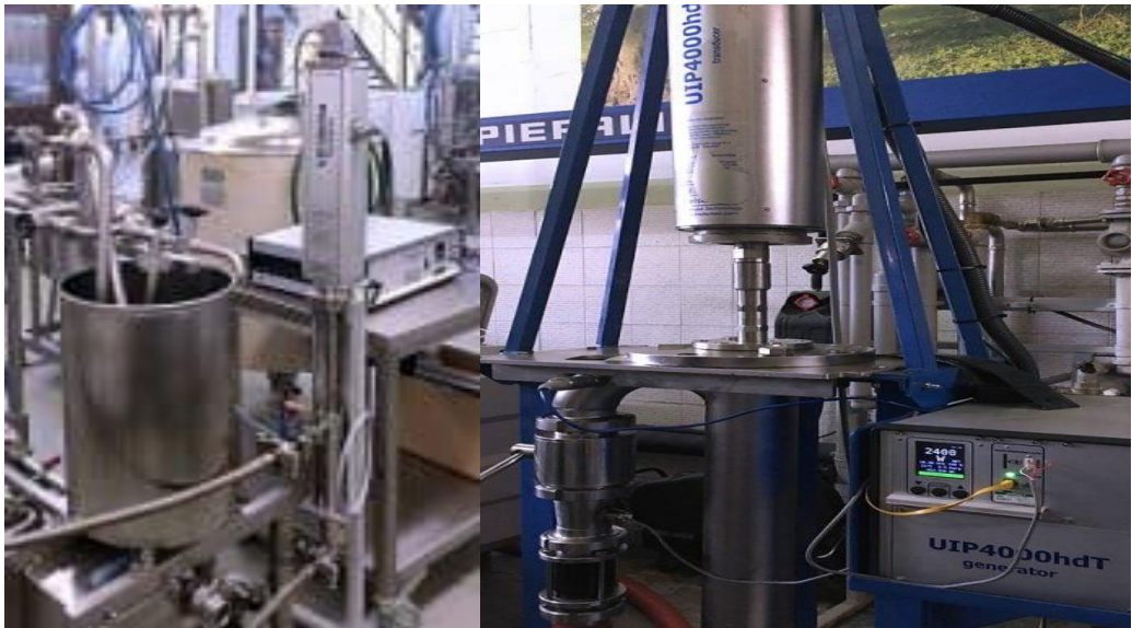
Figure 3 UIP4000hdT (4 kW) ultrasonic extraction system
